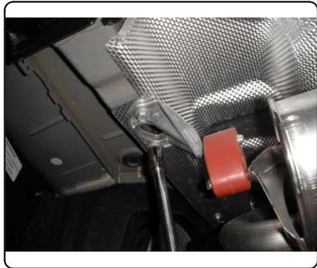
2. Raise hitch into position and temporarily secure to existing weldnuts in the frame rails using (4) M8-1.25 hex bolts and (4) 3/8" conical toothed washers. Using the hitch as a template mark drill location on both sides. Lower hitch and drill holes.
