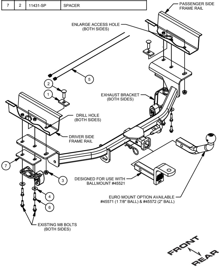
1. Remove (4) bolts and lower the (2) rear exhaust brackets, return bolts to owner.
