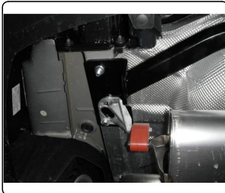
5. Torque all M8 hardware to 23 ft-lbs. Torque all 7/16" hardware to 70 ft-lbs.
